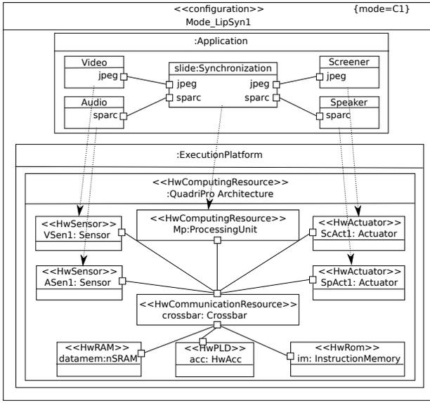
Figure 6. A configuration executed on the processor
