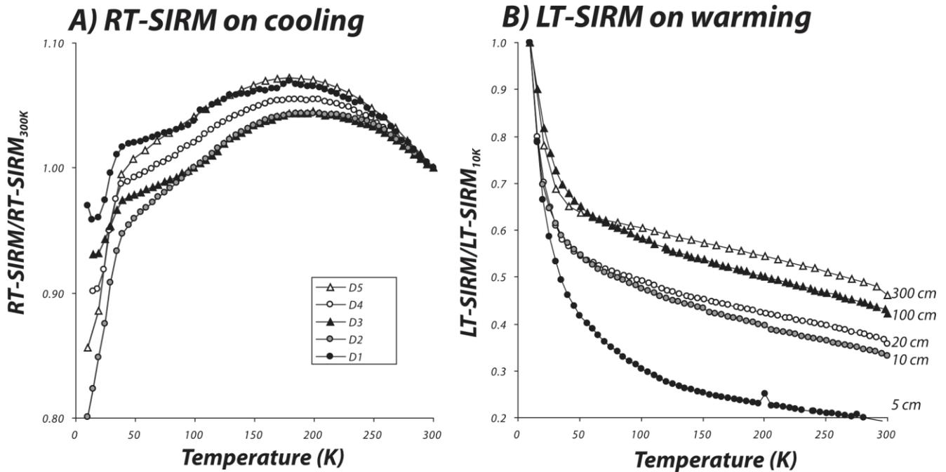
**Figure 7.** Low-temperature magnetic properties of argillaceous rocks along the three-profile next to a 1-m-thick dyke. (a) RT-SIRM. The drop of RT-SIRM near 35 K is the Besnus transition and points for the occurrence of  $>1\mu\text{m}$  pyrrhotite. (b) LT-SIRM curves. The drop from 10 to 300K is varying at a function of distance of the dyke.
