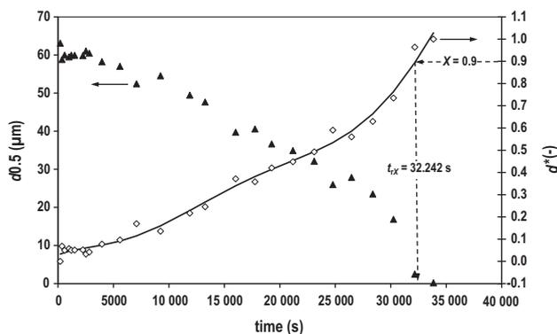
**Figure 2.**  $d_{0.5}$  and  $d^*$  as a function of time during rehydration of MCP at a concentration  $\phi$  of 8% (w/w), 30 °C and 500 rpm. ▲:  $d_{0.5}$  value; ◇: corresponding  $d^*$  value calculated from equation (1); black line stands for polynomial model.
