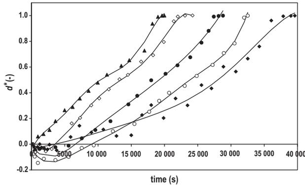
**Figure 3.** Rehydration rate  $d^*$  as a function of time and stirring speed  $N$  (rpm).  $\blacklozenge$ :  $N = 400$  rpm;  $\circ$ :  $N = 500$  rpm;  $\bullet$ :  $N = 600$  rpm;  $\diamond$ :  $N = 800$  rpm;  $\blacktriangle$ :  $N = 1000$  rpm. Black line stands for polynomial model. Fixed  $\phi$  and  $\theta$  values are equal to 4.8% (w/w) and 30 °C, respectively.
