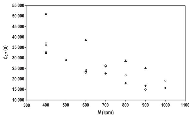
**Figure 5.** Rehydration time  $t_{r0.7}$  as a function of stirring speed  $N$  (rpm) for different solid-liquid concentrations  $\phi$  (w/w). ◆:  $\phi = 4.8\%$ ; ◇:  $\phi = 8\%$ ; ▲:  $\phi = 12\%$ . Fixed  $\theta$  value is equal to  $30^\circ\text{C}$ .
