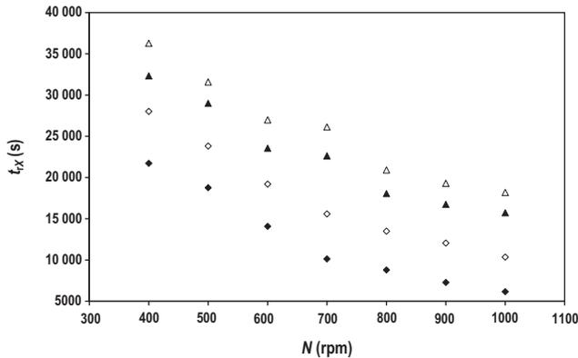
**Figure 4.** Rehydration time  $t_{tX}$  as a function of stirring speed  $N$  (rpm).  $\blacklozenge$ :  $X = 0.3$ ;  $\diamond$ :  $X = 0.5$ ;  $\blacktriangle$ :  $X = 0.7$ ;  $\Delta$ :  $X = 0.9$ . Fixed  $\phi$  and  $\theta$  values are equal to 4.8% (w/w) and 30 °C, respectively.
