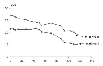
**Figure 3.** C/N ratio decrease during composting of mixtures of poultry manure and exhausted olive cake. Windrow I: 75% poultry manure and 25% exhausted olive cake; windrow II: 25% poultry manure and 75% exhausted olive cake.
