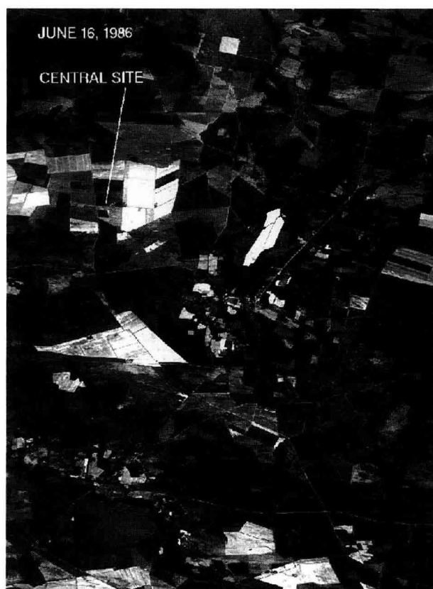
Figure 1. Thermal infrared image from channel 5 (10–11 \mu\text{m} ) of TIMS acquired during the HAPEX-MOBILHY experiment in southwest France in 1986. The data were acquired at an altitude of 6 km with a pixel size of 15 m and cover an area of approximately 10 by 15 km. North is up in the figure. The range of temperature is from 30 ^{\circ}\text{C} for the well-watered vegetation fields and forests to almost 50 ^{\circ}\text{C} for the bare soil fields.
