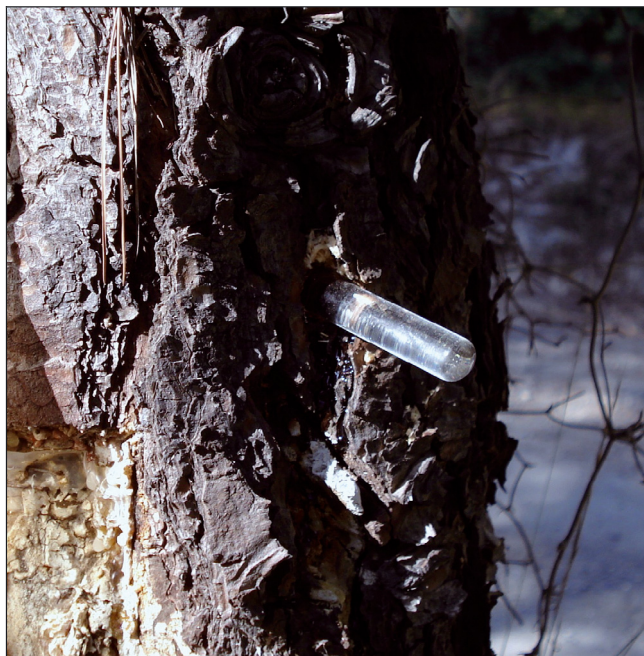
Figure 1. A glass vial full of oleoresin fitted with a slight downwards slope in a P. halepensis trunk. One hole was drilled at breast height on each selected tree.
