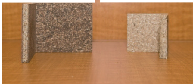
Figure 1. Samples of manufactured particleboards: side and front views.
