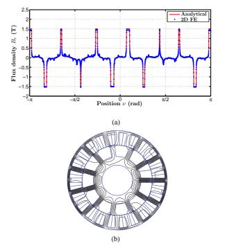
Fig. 20. Magnetic flux density in middle of air-gap  $B_r\left(\nu,\theta\right)|_{r=R_e}$  for a 24-11 slots configuration (3 phase) (with  $\beta_s=0.6,\ L_{ds}=L_{dr}$  and  $n_sI_{exc}=1200A.turn$ ): (a)  $B_r$  distribution for 24-11 slots configuration and (b) the magnetic flux lines with FE software
