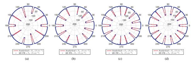
Fig. 17. Magnetic pressure  $P_m(\nu,\theta)|_{r=R_e}$  for a 24 stator slots structure (with  $\beta_s=0.6,\ L_{ds}=L_{dr}$  and  $n_sI_{exc}=1200A.turn$ ): (a) 10 rotor teeth, (b) 11 rotor teeth, (c) 13 rotor teeth and (d) 14 rotor teeth
