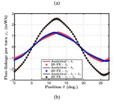
Fig. 11. Flux-linkage (per turn) waveform for a 24 stator slots structure and single-layer winding configuration (with  $\beta_s=0.6$ ,  $L_{ds}=L_{dr}$  and  $n_sI_{exc}=1200A.turn$ ): (a) 10 rotor teeth and (b) 13 rotor teeth
