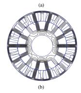
Fig. 22. Magnetic flux density in middle of air-gap  $B_r\left(\nu,\theta\right)|_{r=R_e}$  for a 24-14 slots configuration (3 phase) (with  $\beta_s=0.6,\ L_{ds}=L_{dr}$  and  $n_sI_{exc}=1200A.turn$ ): (a)  $B_r$  distribution for 24-14 slots configuration and (b) the magnetic flux lines with FE software
