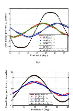
Fig. 14. Flux-linkage (per turn) waveform for a 24 stator slots structure and double-layer winding configuration (with  $\beta_s=0.6,\ L_{ds}=L_{dr}$  and  $n_sI_{exc}=1200A.turn$ ): (a) 11 rotor teeth and (b) 14 rotor teeth
