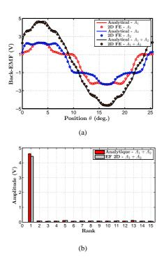
Fig. 16. Back-EMF waveform (a) and its spectra (b) for a 24-14 slots structure and double-layer winding configuration (with  $\beta_s=0.6,\ L_{ds}=L_{dr},\ n_sI_{exc}=1200A.turn$  and  $\Omega=1300rpm$ )
