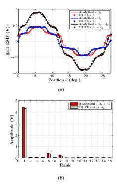
Fig. 13. Back-EMF waveform (a) and its spectra (b) for a 24-13 slots structure and single-layer winding configuration (with  $\beta_s=0.6,\,L_{ds}=L_{dr},\,n_sI_{exc}=1200A.turn$  and  $\Omega=1300rpm$ )
