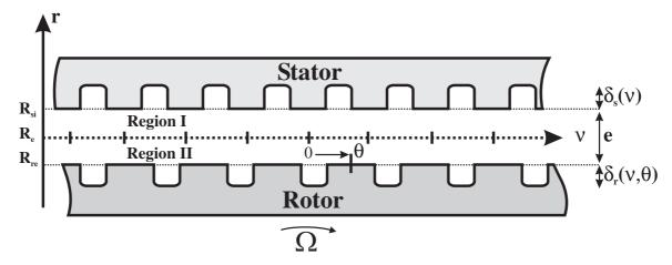
Fig. 4. The extended magnetic circuit of the FE-FS machine in pseudopolar coordinate to evaluate the air-gap permeance  $\Lambda(\nu,\theta)$
