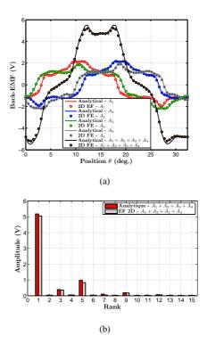
Fig. 15. Back-EMF waveform (a) and its spectra (b) for a 24-11 slots structure and double-layer winding configuration (with  $\beta_s=0.6,\ L_{ds}=L_{dr},\ n_sI_{exc}=1200A.turn$  and  $\Omega=1300rpm$ )
