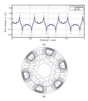
Fig. 9. Magnetic flux density in middle of air-gap  $B_r\left(\nu,\theta\right)|_{r=R_e}$  for a 12-6 slots configuration (single phase) (with  $\beta_s=0.5$ ,  $\beta_r=0.2$  and  $n_sI_{exc}=1200A.turn$ ) in q-axis position and with stator slot wider than rotor tooth: (a)  $B_r$  distribution and (b) the magnetic flux lines with FE software
