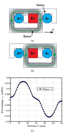
Fig. 1. Flux distribution in stator teeth with field excitation (Region E+) only: (a) Maximum flux-linkage position, (b) minimum flux-linkage position of coil A and (c) evolution of flux-linkage as function of rotor position  $\theta$
