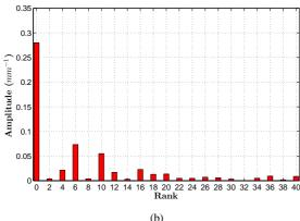
Fig. 7. (a) Evolution of function  $g(\nu,\theta=0)$  (with  $N_s=10,\,N_r=6,\,\beta_s=\beta_r=0.5,\,R_{si}=50mm$  and e=2mm) and (b) spectra of the air-gap permeance  $\Lambda(\nu,\theta)$
