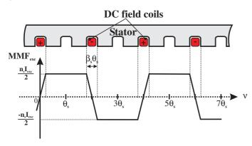
Fig. 3. The Magnetomotive Force created by the DC field coils  $MMF_{exc}(\nu,n_sI_{exc},\beta_s,\theta_s)$
