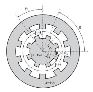
Fig. 2. Doubly-salient geometry of FE-FS machine with  $N_{\rm s}=10$  and  $N_{\rm r}=8$
