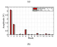
Fig. 12. Back-EMF waveform (a) and its spectra (b) for a 24-10 slots structure and single-layer winding configuration (with  $\beta_s=0.6$ ,  $L_{ds}=L_{dr}$ ,  $n_sI_{exc}=1200A.turn$  and  $\Omega=1300rpm$ )
