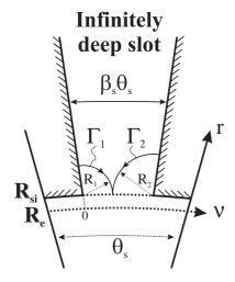
Fig. 5. Magnetic flux-path under an infinitely deep slot
