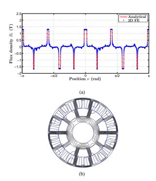
Fig. 19. Magnetic flux density in middle of air-gap  $B_r\left(\nu,\theta\right)|_{r=R_e}$  for a 24-10 slots configuration (3 phase) (with  $\beta_s=0.6,\ L_{ds}=L_{dr}$  and  $n_sI_{exc}=1200A.turn$ ): (a)  $B_r$  distribution for 24-10 slots configuration and (b) the magnetic flux lines with FE software
