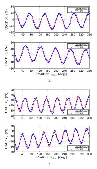
Fig. 18. Evolution of UMF  $(F_x \text{ and } F_y)$  as function of rotor position  $\theta_{elec}$  for a 24 stator slots structure (with  $\beta_s=0.6$ ,  $L_{ds}=L_{dr}$  and  $n_sI_{exc}=1200A.turn$ ): (a) 11 rotor teeth and (c) 13 rotor teeth
