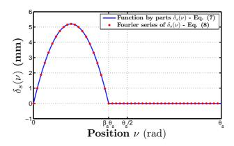
Fig. 6. Comparison between the additional air-gap function  $\delta_s(\nu)$  (Eq. (8)) and its Fourier series development (Eq. (9))
