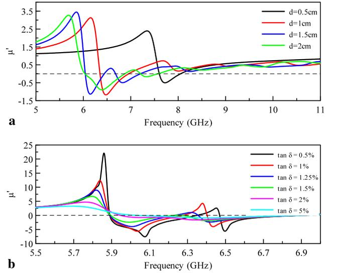
**Fig. 2** (a) Calculated real parts of the magnetic permeability  $\mu'$  for several diameters  $d$  of TiO<sub>2</sub> cylinders varying from 0.5 cm to 2 cm ( $t = 2.8$  mm,  $\epsilon_r \sim 90$ ,  $\tan \delta \sim 5\%$ ). (b) Real parts of the effective permeability  $\mu'$  for  $d = 2$  cm, and  $\tan(\delta)$  varying from 0.5% to 5%
