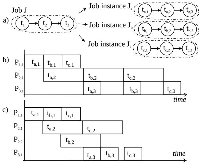
Fig. 4. a) 3 instances of one job  $J$  consisting of three tasks. b) Instances of  $J$  scheduled on architecture shown in Figure 1 a). c) Instances of  $J$  scheduled on architecture shown in Figure 1 b).
