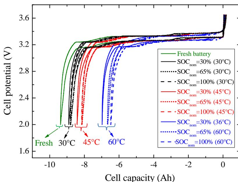
Fig. 8. Discharge/charge PITT between 3.65 V and 2.0 V at  $25^{\circ}\text{C}$  for the fresh cell and for the cells aged under different storage conditions of temperature and SOC, just before the cells are taken apart.
