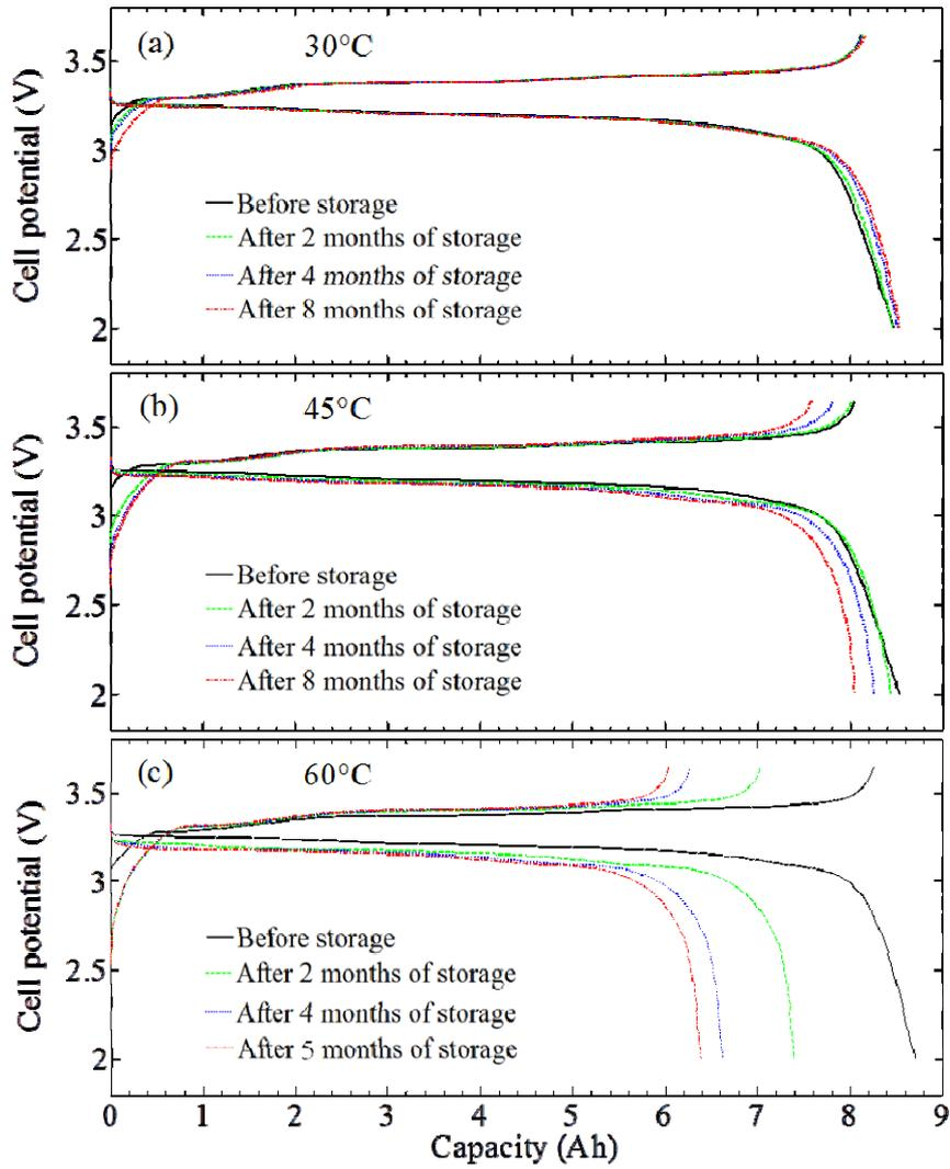
Fig. 1. Charge/discharge profiles measured at  $1C_{nom}$  and  $25^{\circ}\text{C}$  for cells under storage at  $\text{SOC}_{nom}=100\%$  and at temperature (a)  $30^{\circ}\text{C}$ , (b)  $45^{\circ}\text{C}$ , and (c)  $60^{\circ}\text{C}$ .
