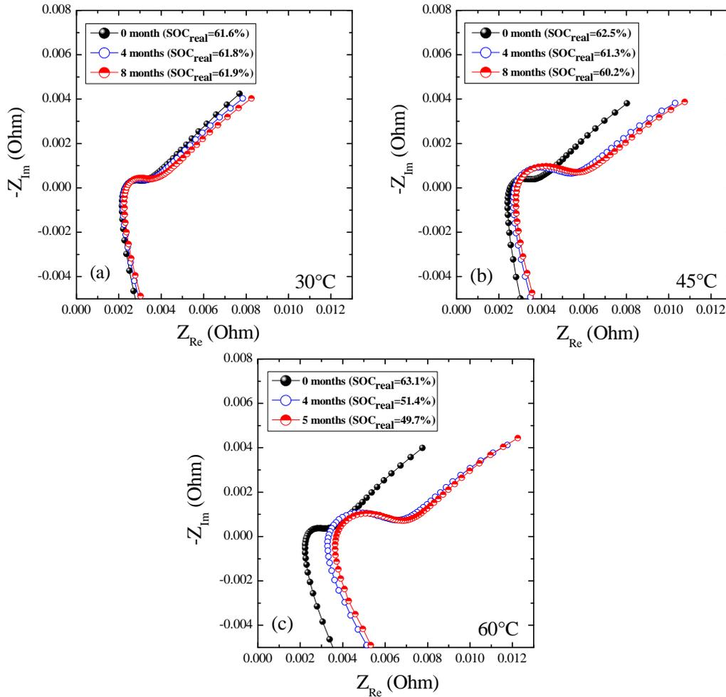
Fig. 5. Impedance spectra measured at 25°C and  $SOC_{nom,ck} = 60\%$  for (a) a cell aged at 30°C and  $SOC_{nom} = 100\%$ , (b) a cell aged at 45°C and  $SOC_{nom} = 100\%$ , (c) a cell aged at 60°C and  $SOC_{nom} = 100\%$ . The real SOC values corresponding to each spectrum are provided in the plot legends.
