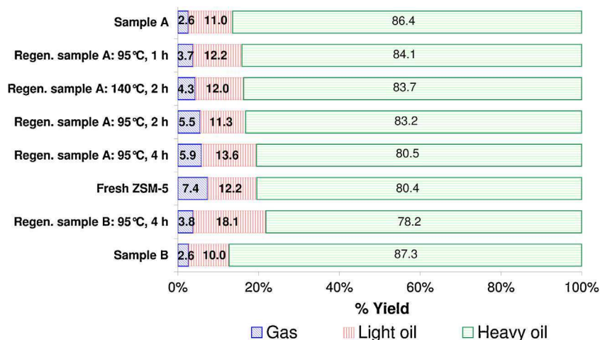
Fig. 11. PMMA degradation yields: distribution of gas, liquid and solid products.
