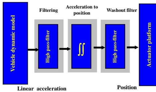
Figure(4) Washout restitution movement algorithm
