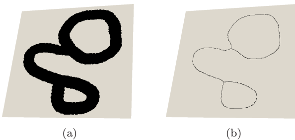
Fig. 3 Illustration of a relation between watersheds and homotopic skeletons. (a): The support of Fig. 1a. (b): A homotopic skeleton of (a).
