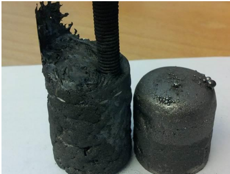
Figure 2. Sample quenched 2 seconds after pure Mg addition (left) and reference sample (right).
