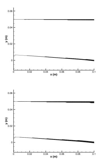
Figure 3: View of the RANS (black) ans LES (white) regions in the mid-span section for the DES computations with  $C_{DES} = 0.65$  (top) and  $C_{DES} = 0.9$  (bottom).
