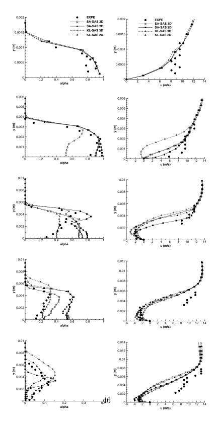
Figure 8: Time-averaged void fraction (left) and longitudinal velocity (right) profiles from station 1 (top) to 5 (bottom), SAS computations.
