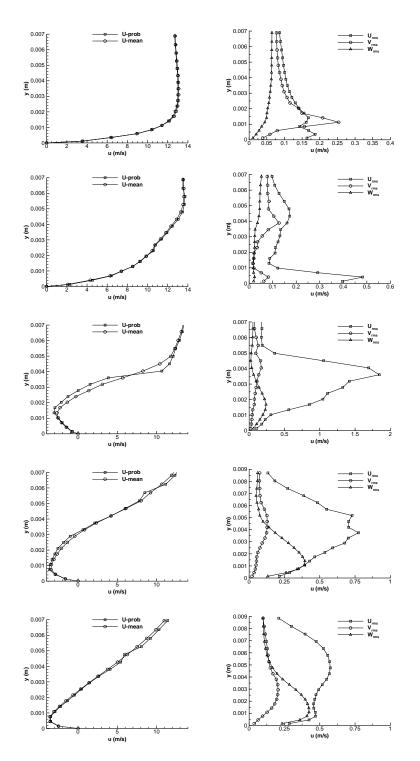
Figure 16: Time-averaged and most probable longitudinal velocity u (left) and RMS of the resolved part of the fluctuating velocities (right) in the n54-span from station 1 (top) to 5 (bottom).
