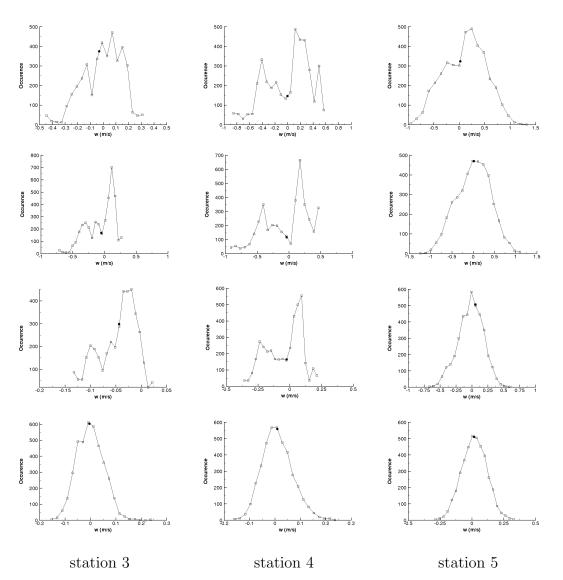
Figure 15: Distribution of the transversal velocity w from station 3 to 5 (left to right) at four distances from the bottom wall: y = 0.7 mm; y = 2 mm; y = 4 mm and y = 8.5 mm (top to bottom). (•) refers to the mean value.
