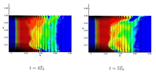
Figure 12: Void fraction and velocity vector at  $\sin_{00}$  different instants, in a cutting plane located at  $y = 10^{-3}$  m.
