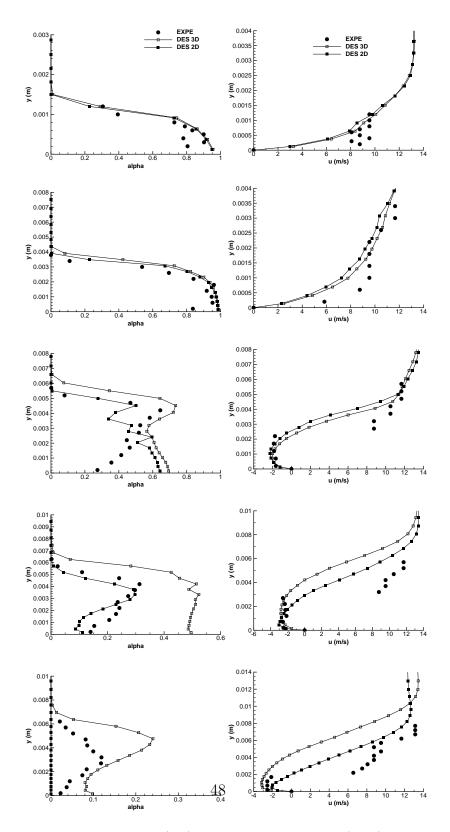
Figure 10: Time-averaged void fraction (left) and longitudinal velocity (right) profiles from station 1 (top) to 5 (bottom), DES computations.
