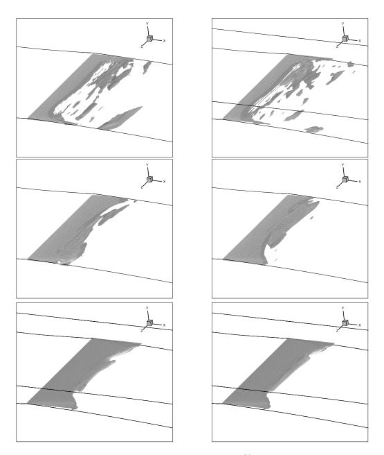
Figure 5: Iso-surface of the void fraction for the value of 60% at two different instants:  $k - \ell$  SAS (top), Spalart-Allmaras SAS (middle) and DES (bottom), 3D computations.
