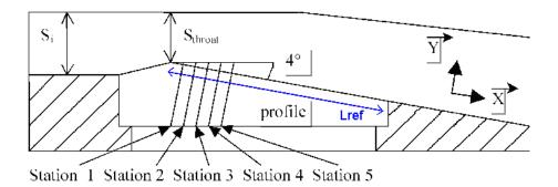
Figure 1: Schematic view of the  $4^{\circ}$  Venturi profile.
