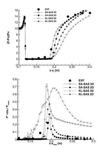
Figure 9: Time-averaged wall pressure (top) and RMS fluctuations (bottom) along the bottom wall, SAS computations.
