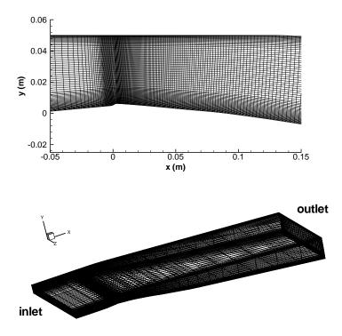
Figure 2: View of the 2D mesh near the Venturi throat and view of the 3D mesh.
