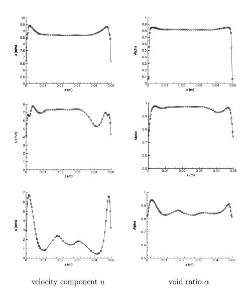
Figure 13: Time-averaged longitudinal velocity (left) and void fraction (right) profiles in the span direction at distance  $y = 10^{-3}$  m and abscissa  $x = 8.3 \, 10^{-3}$  m (top) ;  $x = 2 \, 10^{-2}$  m (middle) and  $x = 2.7 \, 10^{-2}$  m (bottom).
