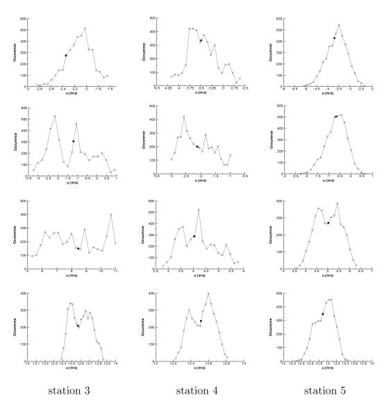
Figure 14: Distribution of the longitudinal velocity u from station 3 to 5 (left to right) at four distances from the bottom wall: y = 0.7 mm; y = 2 mm; y = 4 mm and y = 8.5 mm (top to bottom). (•) refers to the mean value.
