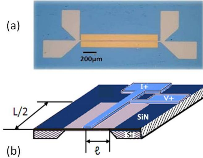
**Figure 1.** Pattern of the heater/thermometer line on the SiN membrane (a). Cross section schematic of the Völklein geometry (b). The width of the heater/thermometre line is typically  $20\mu\text{m}$ , the width of the membrane is equal to  $200\mu\text{m}$  and the length (1.0mm).
