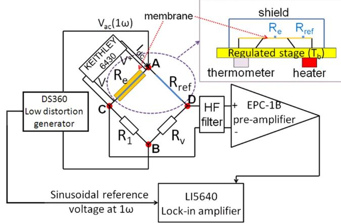
**Figure 3.** Schematic of the electrical measurement system including HF filter, preamplifier and lock-in amplifier. A, B, C and D represent the nodes of the Wheatstone bridge. The  $V_{3\omega}$  is measured between C and D. The transducer is referred as  $R_e$  and the reference resistance as  $R_{ref}$ . The insert presents a schematic of the membrane fixed on the temperature regulated stage covered by the thermal copper shield.
