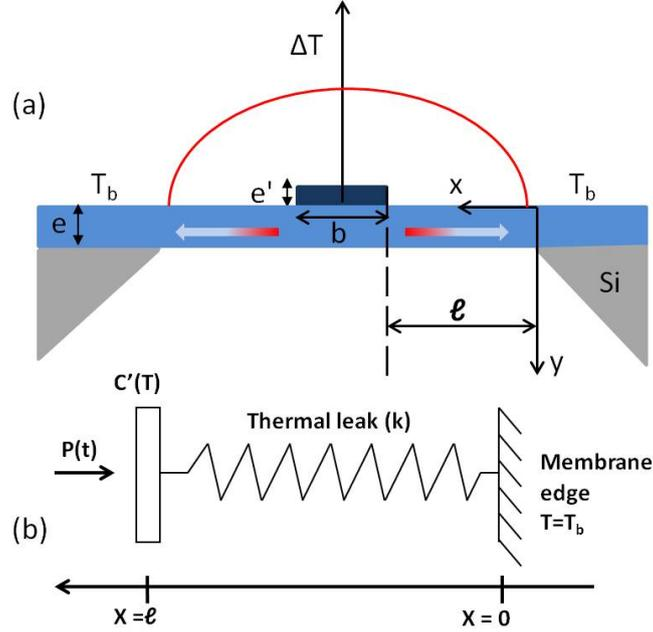
**Figure 4.** (a) Schematic of the membrane on which the NbN transducer is deposited.  $e$  is the thickness of the membrane and  $e'$  the thickness of the NbN transducer. (b) Schematic of the thermal system.
