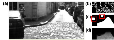
Fig. 6 – (a) Original image after sky removal and its Otsu's result in (c); (b) Canny edge detection result; (d) A multimodal 2D drivability free-area by considering the drag process.
