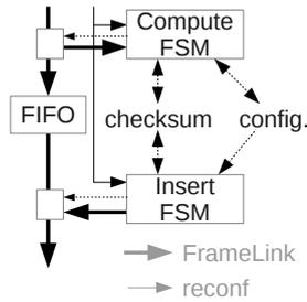
**Figure 4: Architecture of the *checksum* modifier block**
