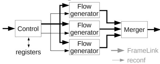
**Figure 2: Architecture of the hardware generator block**
