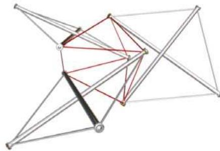
Figure 3 : Simplex generation by assembly of three "X" components
