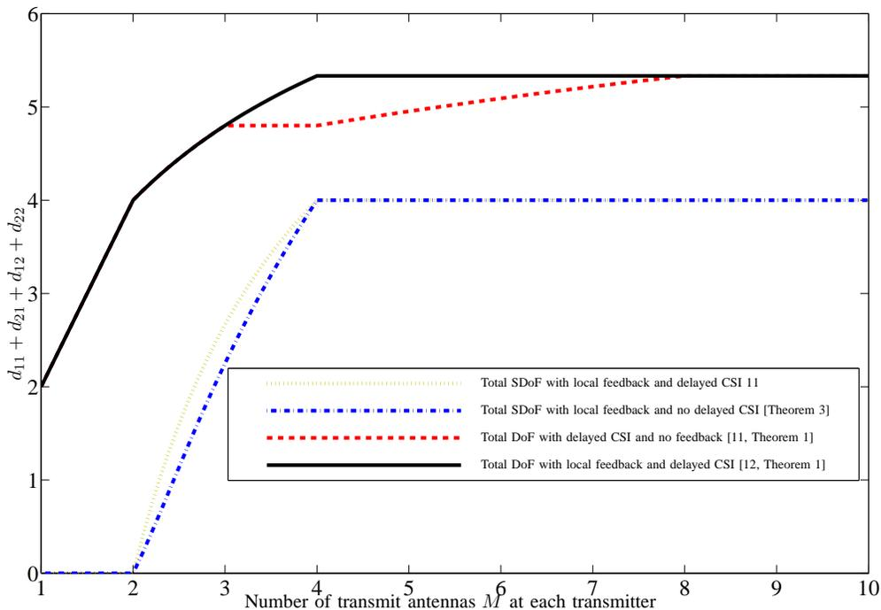
Fig. 7. Total secure degrees of freedom of the MIMO  $(M, M, N, N)$ -X channel, as a function of the number of transmit antennas  $M$  at each transmitter, for a fixed number  $N = 4$  of receive antennas at each receiver.
