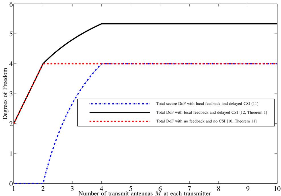
Fig. 3. Total secure degrees of freedom of the  $(M, M, N, N)$ -MIMO X-channel as a function of the number  $M$  of transmit antennas at each transmitter, for a fixed number  $N = 4$  of receive antennas at each receiver.
