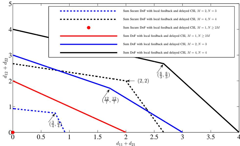
Fig. 5. Sum SDoF and sum DoF regions of the  $(M, M, N, N)$ -X channel with local output feedback and delayed CSI, for different antennas configurations.
