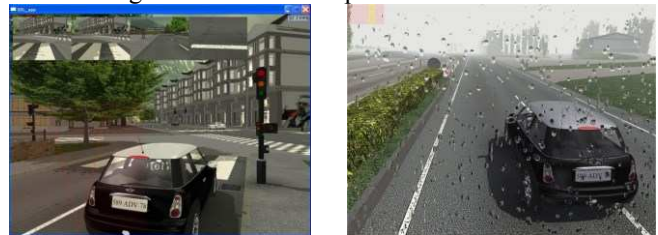
Figure 3: SiVIC platform: Multi-sensors management in a complex environment, and degraded weather conditions.
