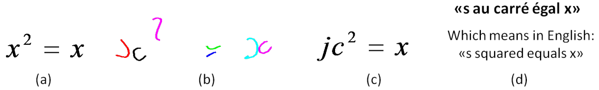
Figure 7. Real example of a contribution of the bimodal processing; (a) the ground-truth ME, (b) its handwritten version, (c) the recognized result without fusion, (d) the automatic transcription of its spoken description
