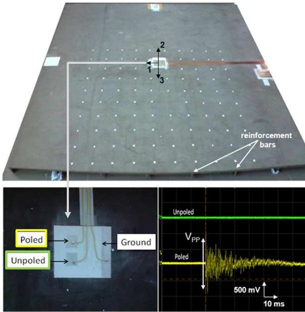
**Figure 3.** Image of the aeronautical CFRC. The white points indicate the 100 points of the databank forming a  $90 \times 90 \text{ cm}^2$  area used for location. Image of the as prepared piezoelectric sensors sprayed on a  $1.6 \times 1.6 \text{ m}^2$  and 2 cm thick aeronautical CFRC. An unpoled sensor was taken as reference. The electrical response of an impact performed on an aeronautical CFRC measured by the poled and unpoled sensors.
