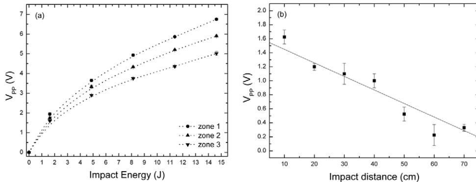
**Figure 4.** (a) Electrical response  $V_{PP}$  of the piezoelectric paint versus the impact energy for an impact at 35 cm from the sensor. The direction 1 corresponds to the direction orthogonal to the reinforcement bars and directions 2 and 3 are parallel to the reinforcement bars. (b) Electrical response  $V_{PP}$  of the piezoelectric paint versus the distance between the impact and the sensor for an impact energy of  $E = 1.6 \text{ J}$  in direction 3.
