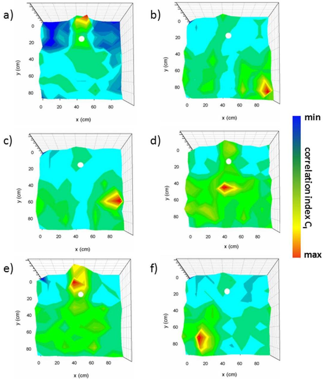
**Figure 5.** (a)–(f) Real time impact location using the cross correlation technique. The red color reports the maximum correlation index and the white circle shows the active sensing coating location.
