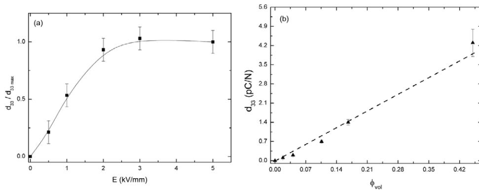
**Figure 2.** (a) The piezoelectric strain constant  $d_{33}$  of PU/BaTiO<sub>3</sub> 300 nm composite with  $\phi = 12\%$  versus the electric field applied during the poling process at  $T = 80^\circ\text{C}$  for 30 min; and (b) the piezoelectric strain constant  $d_{33}$  versus the volume fraction of BaTiO<sub>3</sub> filler.
