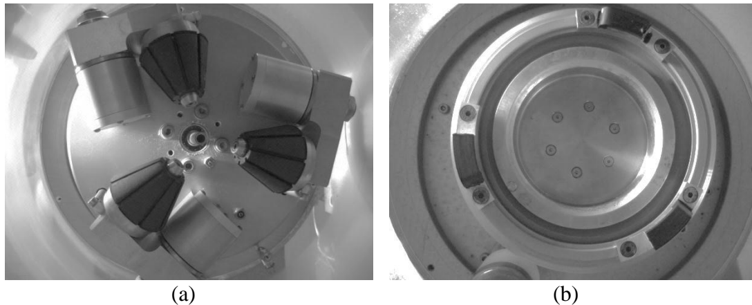
Figure 2. (a) Three rubber conical polishing rollers; (b) Three rubber slider pads
