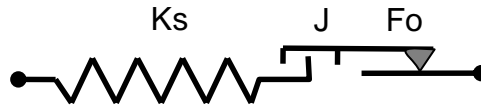
Figure 2 – Dry friction element with free play, used to simulate the side bearers
