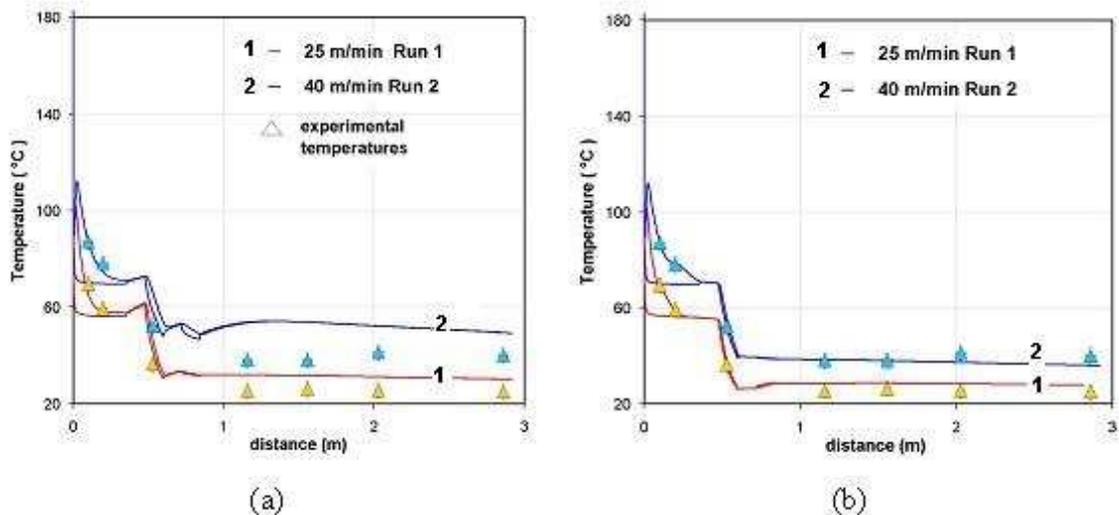
Figure 1: Computed temperature field along the process: (a) without influence of the stretching step on crystallization kinetics, (b) with influence of the stretching step
