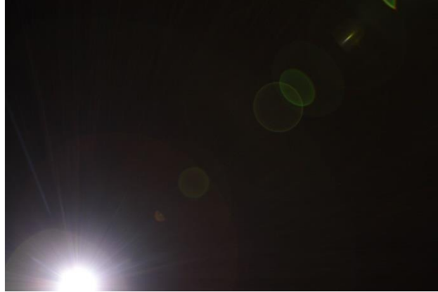
Fig. 3. Demonstration of inner lens reflection artifacts acquired by camera
