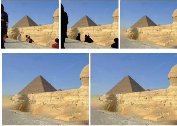
Fig. 4. Large holes inpainting on an image of Gizeh pyramid using a window 61 and patch 13 and ten iterations. From left to right, the original image, the corrupted image, the result of a local inpainting and our nonlocal inpainting results for p = 2 and p = 1 .
