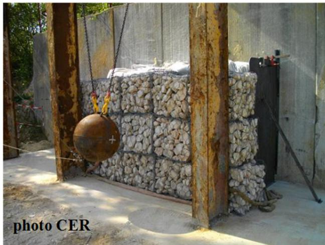
Figure 2 Tested sandwich structure.
