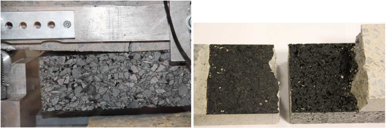
Figure 9. Typical debonding fracture aspect of Type II specimen (II-PT-2-2)
