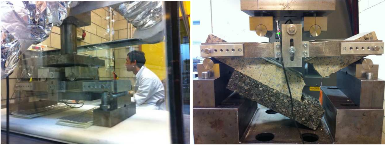
Figure 6. (a) Four-point bending test arrangement (b) First debonding observations of Type I specimen (I-PT-2-3 under load controlled condition 100N/s)
