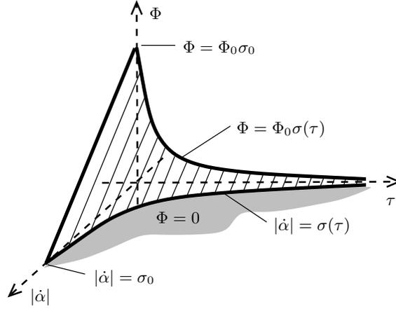
Figure 2: Perspective view of the function  $(|\dot{\alpha}|, \tau) \in [0, +\infty]^2 \rightarrow \Phi(|\dot{\alpha}|, \tau)$  in the case  $a = 0$ . The value  $\sigma_0$  corresponds to  $\sigma_0 = \sigma(0) = \frac{b}{\tau_0^c}$  (in the case  $a = 0$ ). The function  $\Phi$  is identically zero, except for the dashed area, where it is linear. The introduction of  $\tau_0 > 0$  makes it bounded from above by  $\sigma_0$ .
