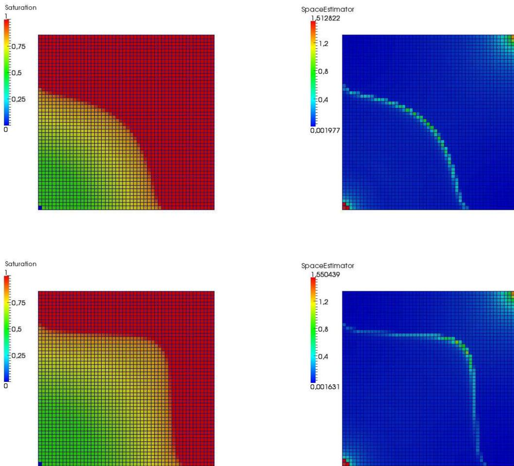
Figure 5: Liquid saturation (left) and distribution of the spatial estimators (right) for the adaptive resolution at times  $7.8 \times 10^7$ s and  $2.1 \times 10^8$ s, the test case of Section 5.2
