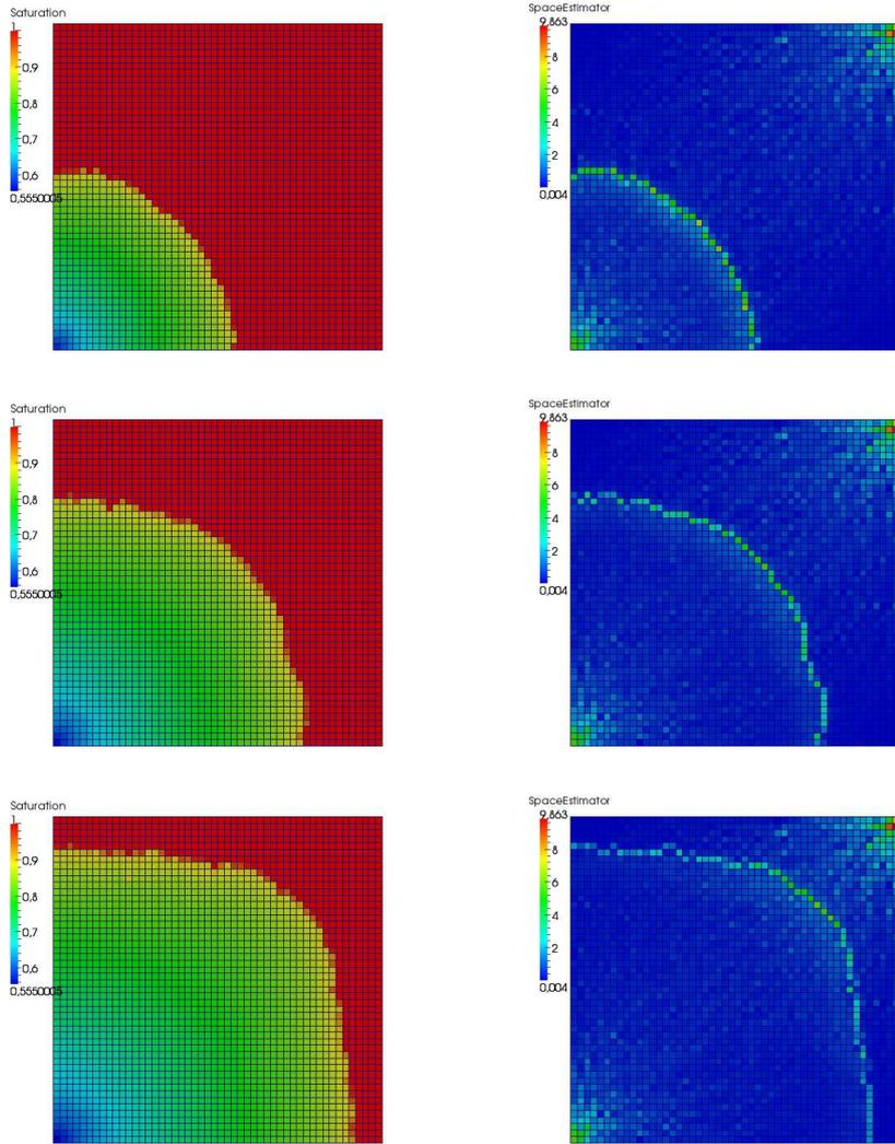
Figure 9: Liquid saturation (left) and distribution of the spatial estimators (right) for the adaptive resolution at times  $5.2 \times 10^7$ s,  $1.04 \times 10^8$ s, and  $1.6 \times 10^8$ s, the test case of Section 5.3
