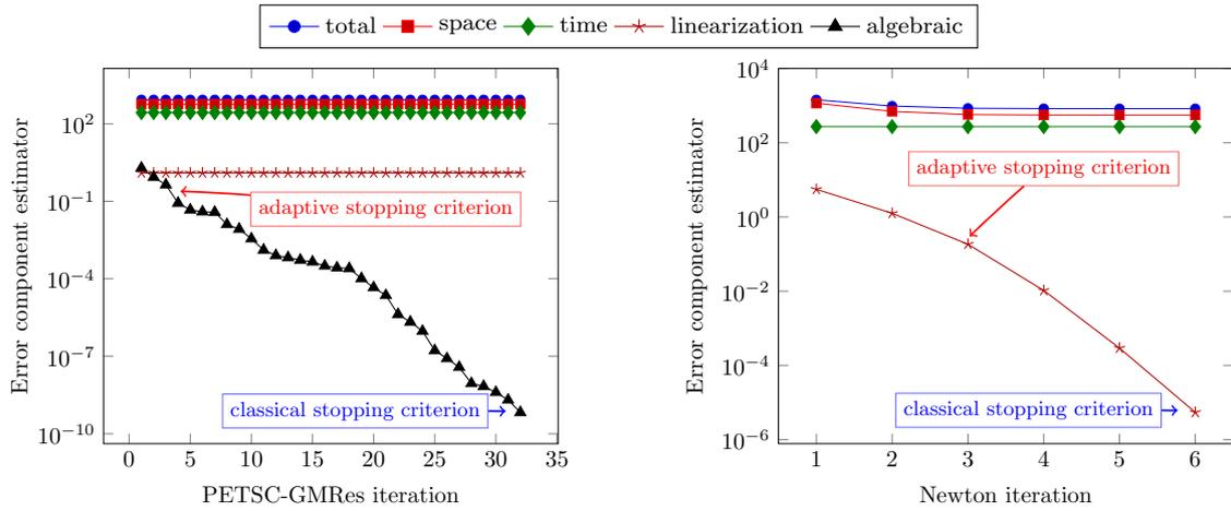
Figure 2: Evolution of the spatial, temporal, linearization, and algebraic error estimators (4.20) for a fixed mesh at time  $1.04 \cdot 10^6$ s, as a function of GMRes iterations on the first Newton iteration (left) and of Newton iterations (right)
