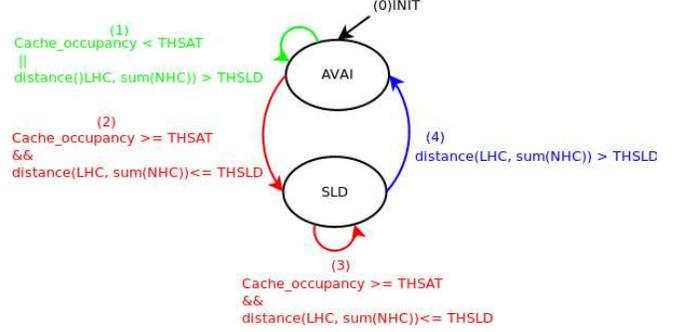
Figure 2. State machine of Data Sliding mechanism
