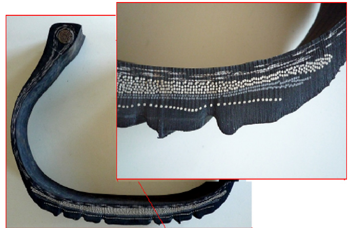
Fig. 3. Layout of the composite structure.
