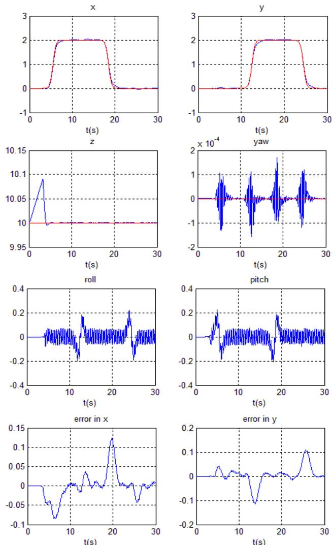
Fig. 4. Event triggered  $i$ -PID control of quadrotor
