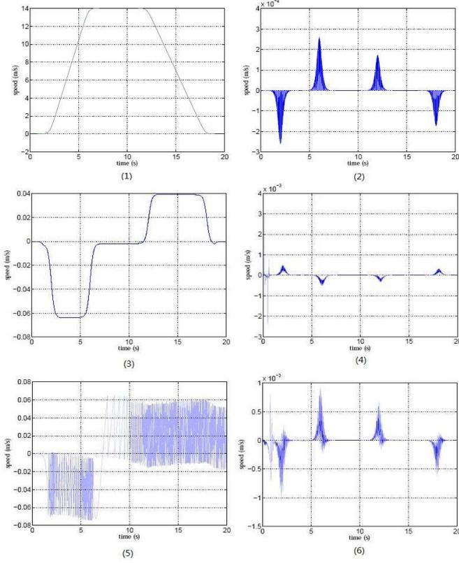
Fig. 1. (1) Reference trajectory. (2) Tracking errors of ideal flatness based control. (3) Tracking errors of time triggered PI control. (4) Tracking errors of time triggered  $i$ -PID control. (5) Tracking errors of event triggered PI control. (6) Tracking errors of event triggered  $i$ -PID control.
