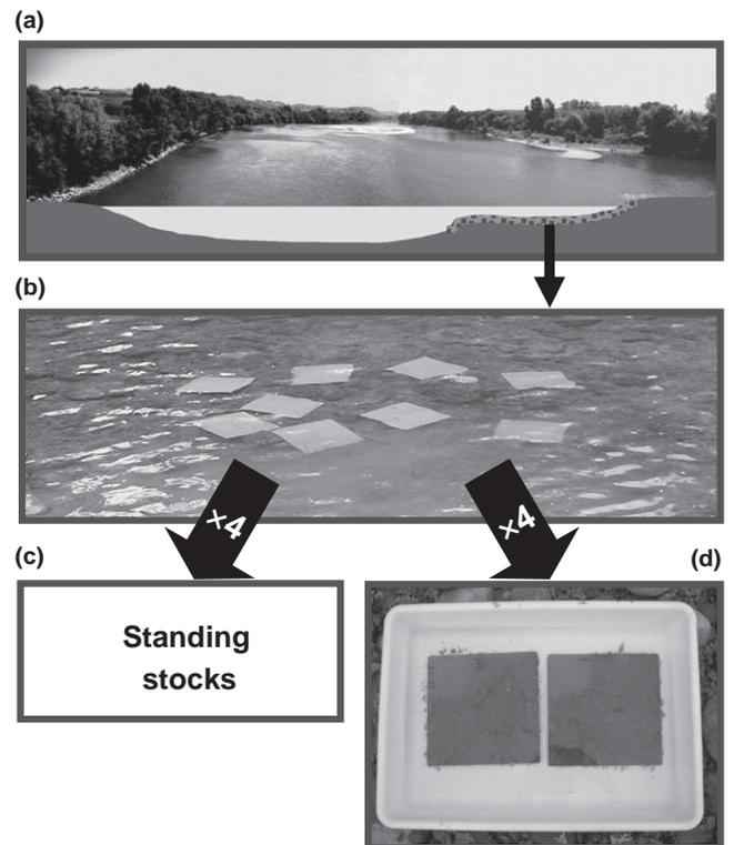
**Fig. 1** Experimental design: (a) Cross-section view of the Garonne River at the study site. (b) Ceramic tiles lying on the streambed before colonisation by biofilm (20 July 2009). After 2 months of colonisation: (c) biofilm was gathered from four tiles to estimate initial standing stocks, and (d) biofilm from four other tiles was labelled with  $\text{NaH}^{13}\text{CO}_3$  solution for 3 h.
