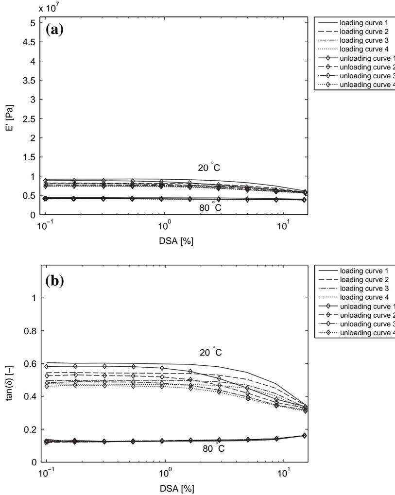
**Fig. 2.**  $E'$  (a) and  $\tan \delta$  (b) of unfilled nitrile rubber vs. DSA during cyclic sweeps at both ambient temperature and 80 °C under tensile loading conditions.
