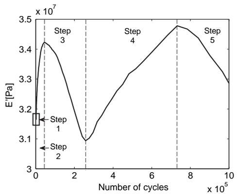
**Fig. 6.** Elementary steps of a fatigue test illustrated at 2.8% DSA at ambient temperature.
