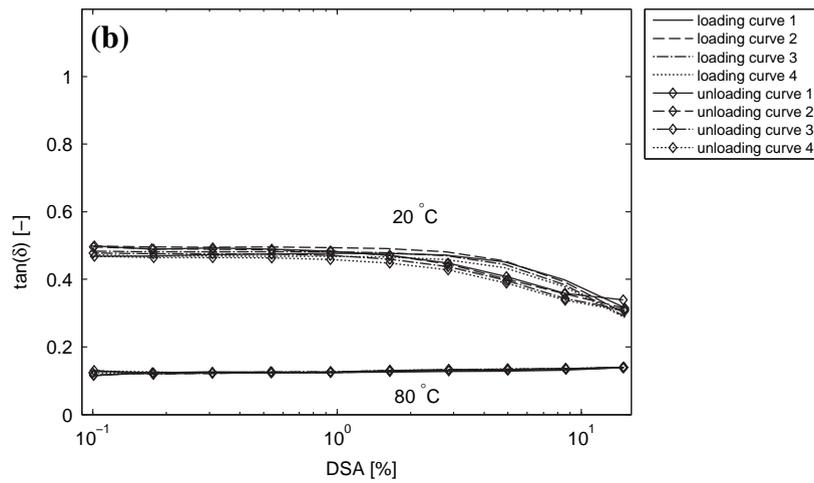
**Fig. 4.**  $E'$  (a) and  $\tan \delta$  (b) of unfilled nitrile rubber vs. DSA during cyclic sweeps at both ambient temperature and 80 °C under compressive loading conditions.
