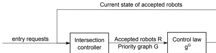
Figure 5: Scheme of the overall coordination system.
