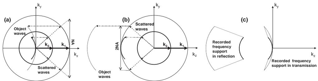
**Figure 10.** TDM with illumination wavelength variation: construction of the object frequency support in transmission and reflection modes.
