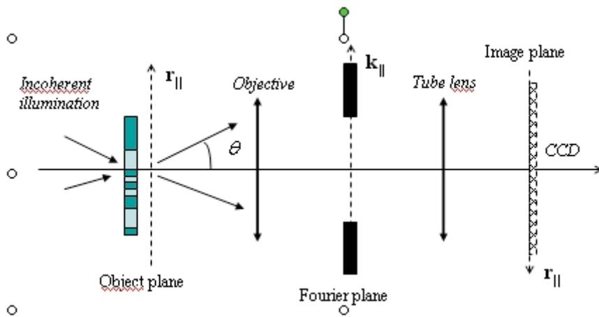
**Figure 4.** Principle of detection of the diffracted wave in a classical transmission microscope.
