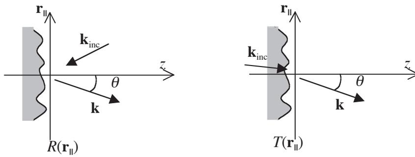
**Figure 2. Different imaging configurations.** Left :Reflection configuration, the object is defined by its reflectance  $R(r_{\parallel})$ . Right transmission configuration, the object is defined by its transmittance  $T(r_{\parallel})$ .
