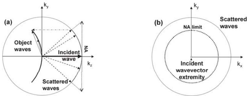
**Figure 5.** Construction of the set of object detected frequencies in the Fourier space in the case of digital holographic microscopy. (a): longitudinal view, and (b): transverse view.
