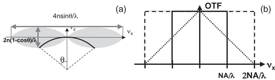
**Figure 7.** (a) Comparison of frequency supports for holography (solid line) and TDM in transmission with illumination rotation (in grey), longitudinal view. (b): Comparison of Optical Transfer Functions for incoherent transmission microscopy (dotted line), holographic microscopy (solid line), and transmission TDM (dashed line). Note that in (b), for the sake of simplicity, the geometry is assumed to be invariant along the  $y$  axis.
