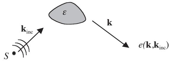
**Figure 1.** A plane wave with wavevector  $\mathbf{k}_{inc}$  illuminates an object characterized by its relative permittivity  $\epsilon$ . The detected diffracted field in the direction  $\mathbf{k}$  is given by  $\mathbf{e}(\mathbf{k}, \mathbf{k}_{inc})$ .
