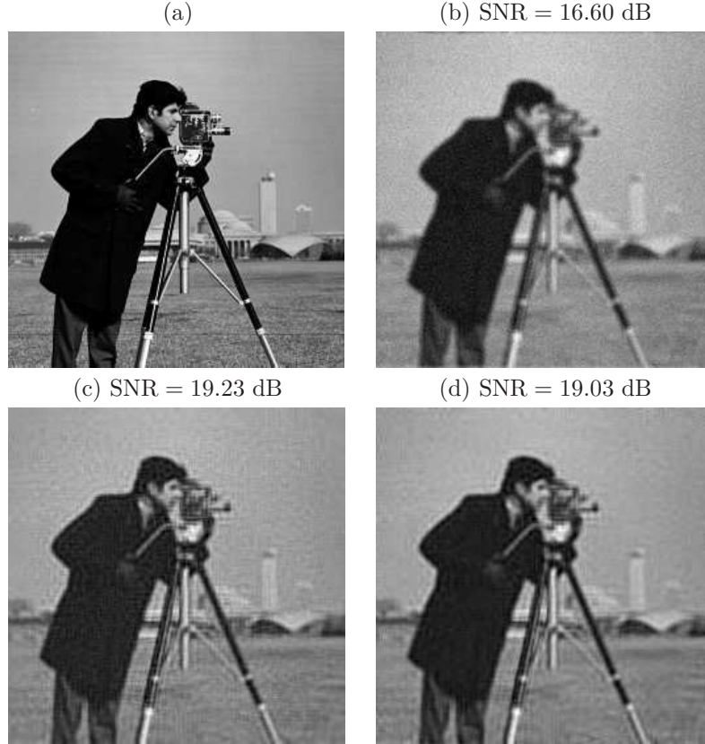
Figure 1. Original image (a), degraded one (b) and restored images using AA (c) and SA (d).
