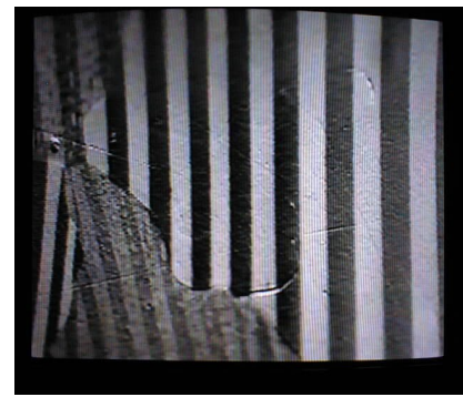
Fig.3: Domain structure in a Fe-Si grain oriented steel sheet obtained by magneto-optical Kerr effect.
