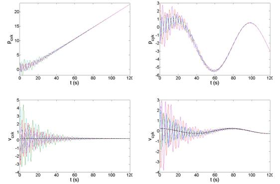
Fig. 3. Evolution of the centers' positions and velocities  $\mathbf{p}_{ck} = (p_{cxk}, p_{cyk})^T$ ,  $\mathbf{v}_{ck} = (v_{cxk}, v_{cyk})^T$  corresponding to the previous simulation of five agents shown in Fig. 2.
