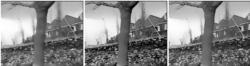
Fig. 2. Illustration of our three denoising methods with parameters p = 2 , \lambda = 0 and h = 30 after ten iterations. (a) original image; (b) noisy image; from left to right: local, nonlocal and optimized nonlocal results.
