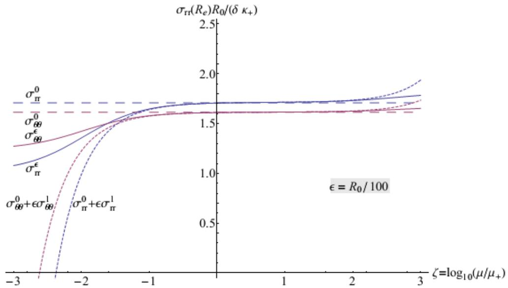
**Figure 2.** Bonding of two spheres: comparative plots of the radial and circumferential stresses on the external surface calculated from the exact three-phase solution, the perfect (order 0) and the imperfect (order 1) interface approximations.
