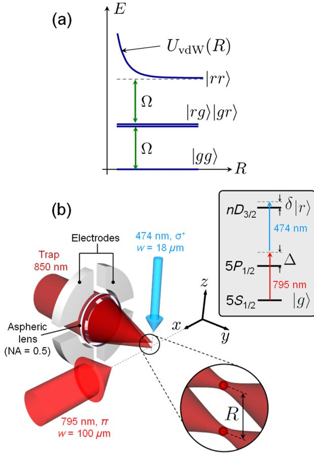
FIG. 1 (color online). (a) Principle of the Rydberg blockade. The single-atom Rabi frequency is  $\Omega$ . (b) Experimental setup. Two single atoms are trapped in microscopic optical traps separated by  $R$ . Eight electrodes (four of which, facing the ones displayed here, are not shown) provide electric field control. Inset: two-photon excitation scheme (the intermediate-state detuning is  $\Delta \simeq 2\pi \times 740$  MHz).
