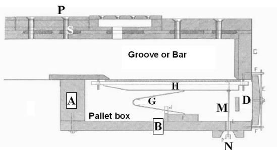
Figure 1: Cross section of a bar (groove) and slider windchest adapted from Audsley Figure CLIX. The significant parts are described in the text
