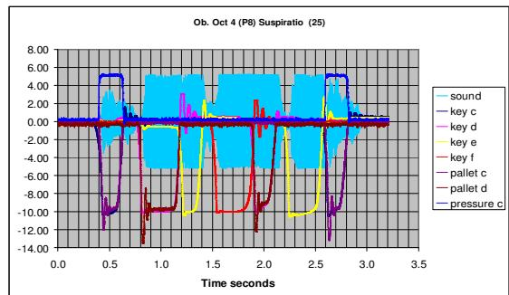
Figure 7: Graph showing the key and pallet movements. pressure in the groove and sound recording for a theme played with Spiratio Rhetorical Figure. Örgryte Church
