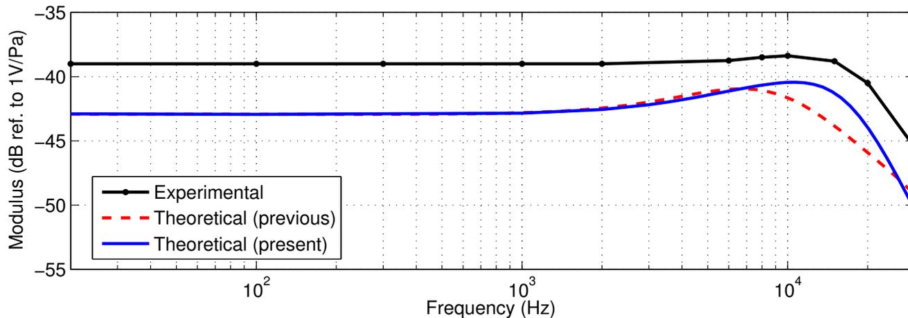
Figure 5: Sensitivity of the microphone vs frequency.
