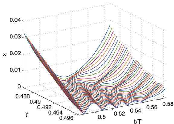
Figure 2: A few periodic solutions on the branch near  $\gamma = 0.48$ : zoom on the part of the period where the beating occurs. Each curve shows the time series of the reed position  $x$ . Computed with HBM using 300 harmonics on a simplified model with a single acoustic mode.
