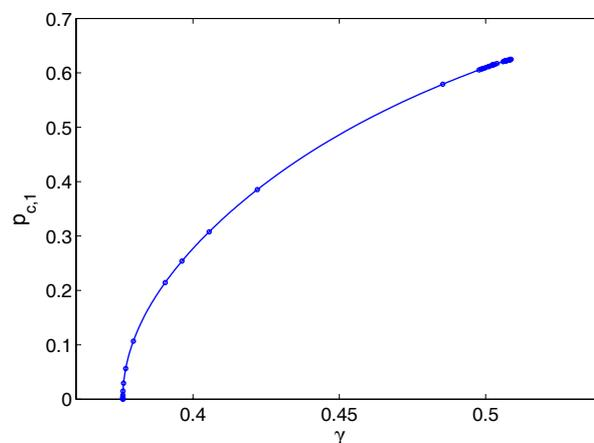
Figure 1: First periodic regime of the clarinet: the curve represents the branch of periodic solutions that destabilizes the static regime at the oscillation threshold ( $\gamma_{th} = 0.373$ ). Computed using ANM (power series order: 20) and HBM (50 harmonics). (—): first harmonic's cosine coefficient of the pressure  $p_{c,1}$  as a function of the blowing pressure  $\gamma$ . The circles mark the beginning of each continuation step.
