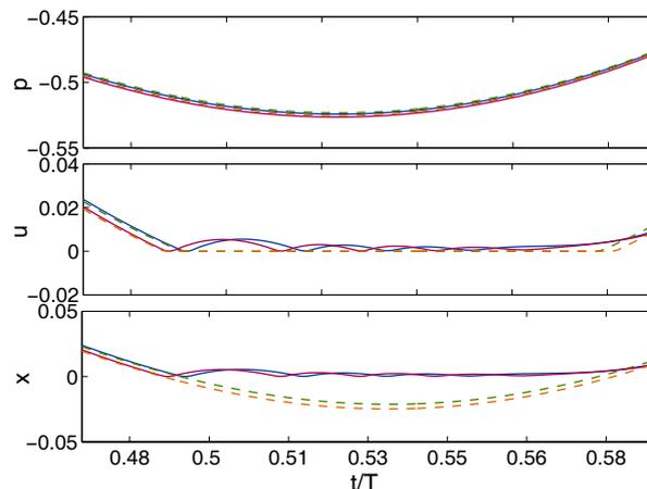
Figure 3: Comparison between a model with regularised contact (—) and a model with a phantom reed (- - -): partial time series of the mouthpiece pressure  $p$ , the volume flow  $u$  entering the reed channel, and the reed tip position  $x$  when the beating occurs. corresponding values of  $\gamma$  are between 0.494 and 0.496.
