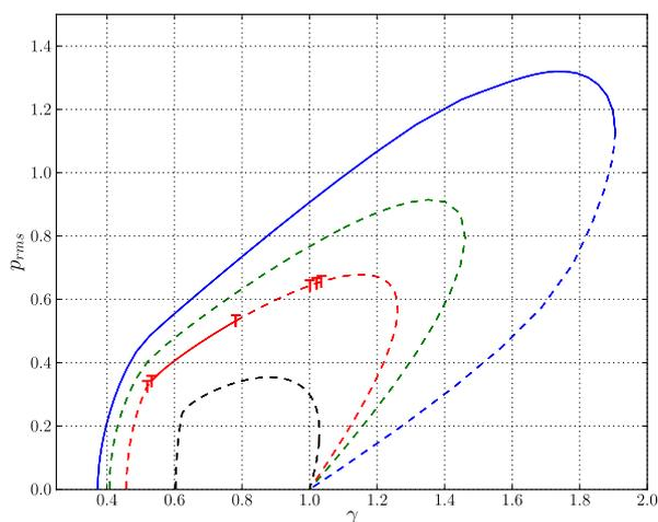
Figure 6: Bifurcation diagram: periodic regimes of the clarinet. Each curve represents a branch of periodic solutions. Plain lines denote stable parts, and unstable ones are denoted by a dotted line. Computed using the AUTO software.
