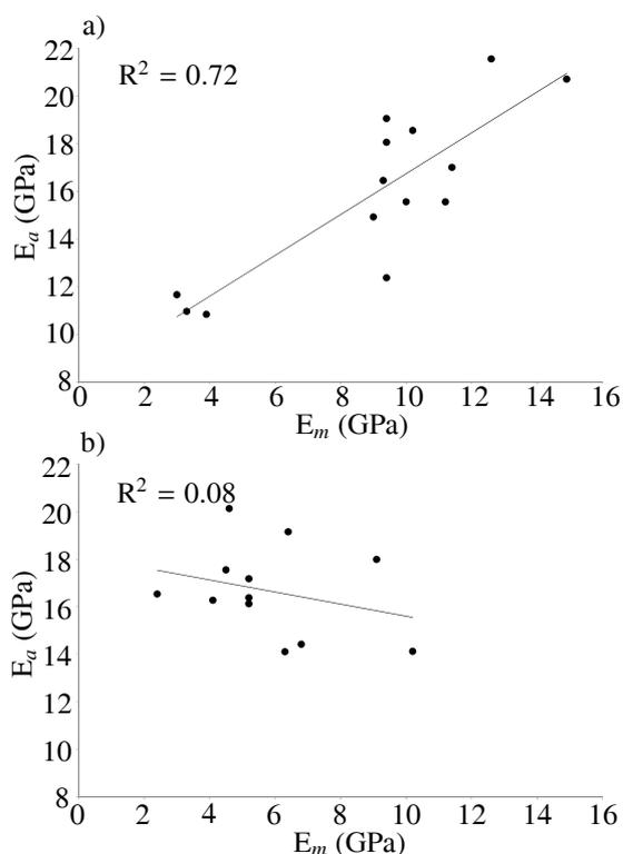
Figure 3: Correlation between Young's modulus measured by 3-point bending test (longitudinal direction) and Young's modulus measured by ultrasound (transverse direction): a) children group; b) senior group
