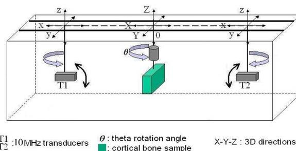
Figure 1: Ultrasonic experimental setup
